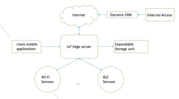
Figure 1. High level design for IoT Edge server
